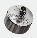
suitable for solenoid system .032 and .012 End position detection sensor Stainless steel 1.4301 / 1.4105 Housing material 12-24V DC Supply voltage Ambient temperature -40 °C to +80 °C M12x1 5-pin Electrical connection Thread / connection G<sup>1</sup>/<sub>8</sub> (others on request)
