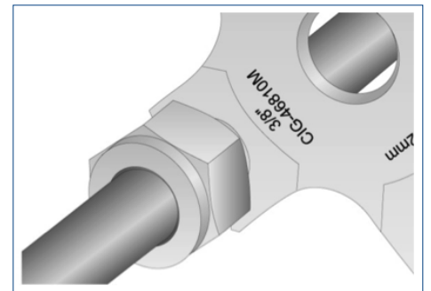
Go Insufficiently tightened
