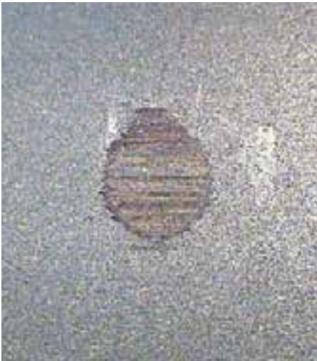
Figure 4 Typical wear dimple after 15 min
