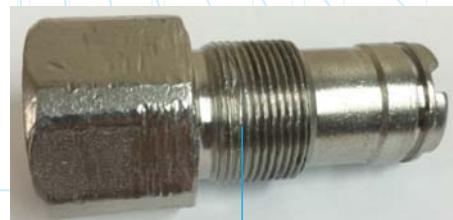
Damage to threads on SDX III Nozzle
